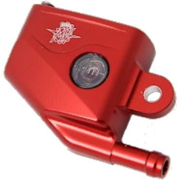
**Rear brake oil tank 20 ml** with level porthole machined from solid by CNC machines with subsequent red surface anodization which ensures quality and durability
