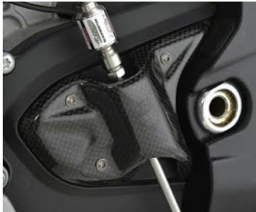
**Sprocket cover in carbon fiber**
